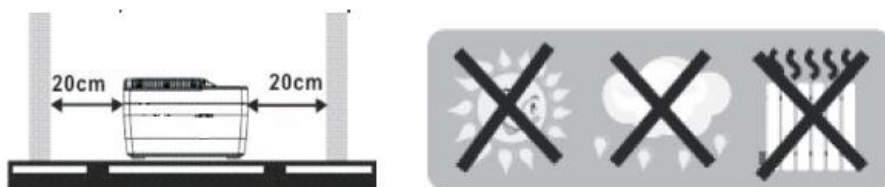
Figure 1. Placing of the UPS
