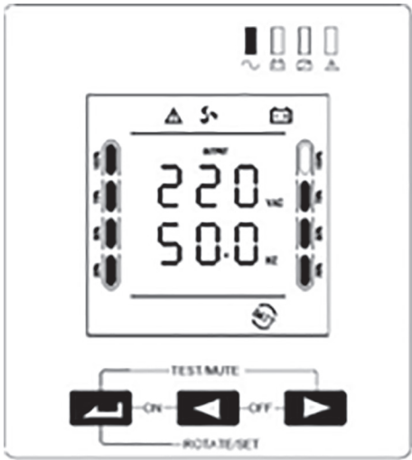
Figure 12. Display of the UPS
