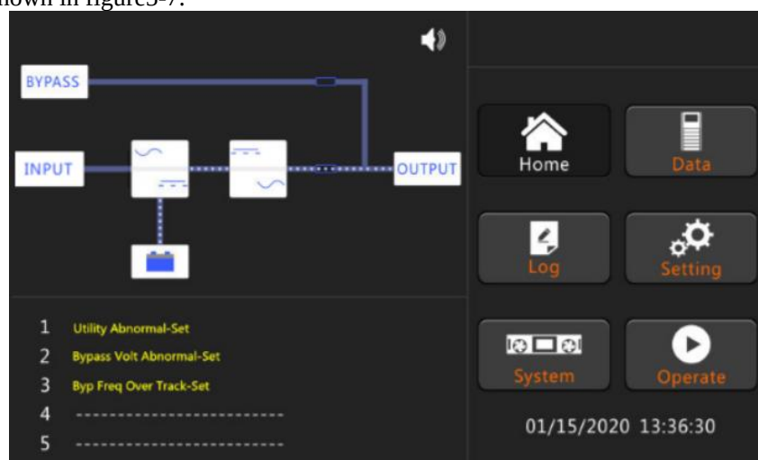
Figure5.7 Energy flowing diagram of the start completed from batteries
