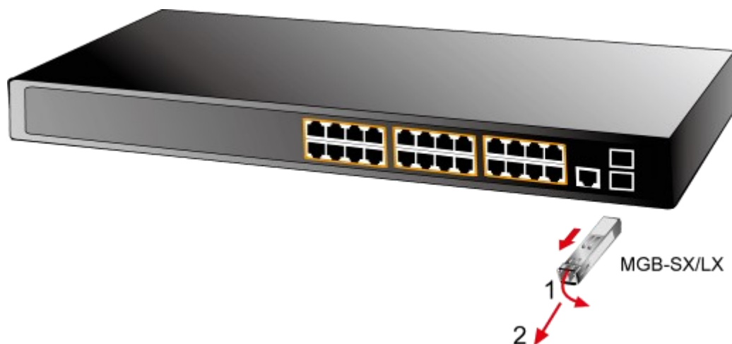
Figure 2-1-8: How to Pull Out the SFP Transceiver
