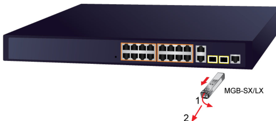
Figure 2-8: How to Pull Out the SFP Transceiver
