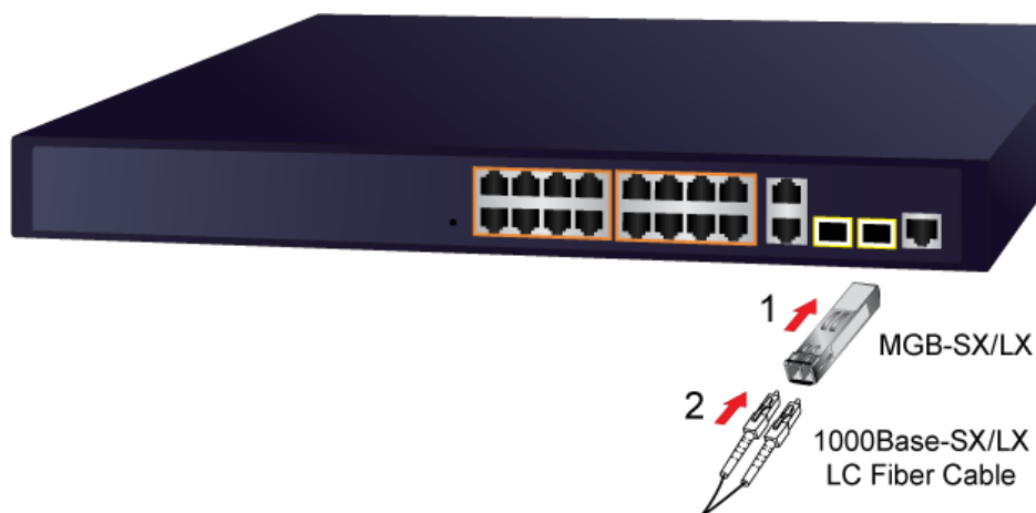
Figure 2-7: Plug-in the SFP Transceiver
