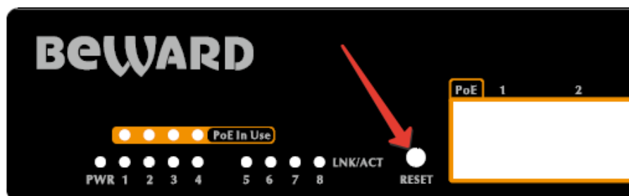
Figure 2-2 Reset button of STW-8P4
