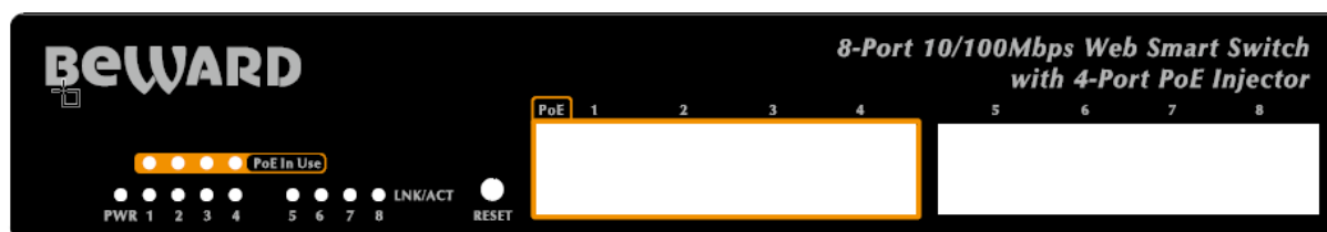
Figure 2-1 STW-8P4 Switch front panel
