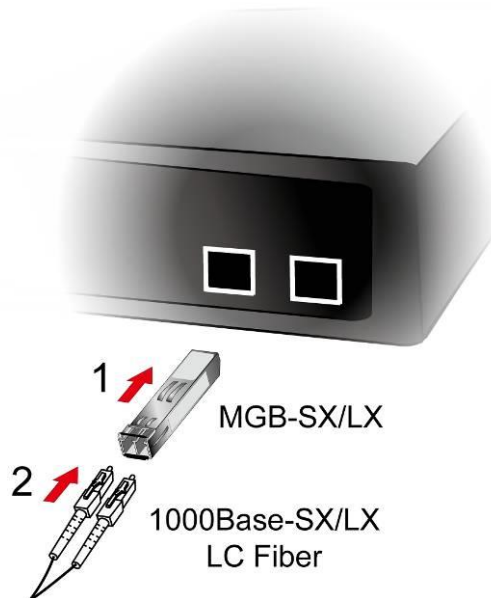
Figure 2-2-1 Plug in the SFP transceiver
