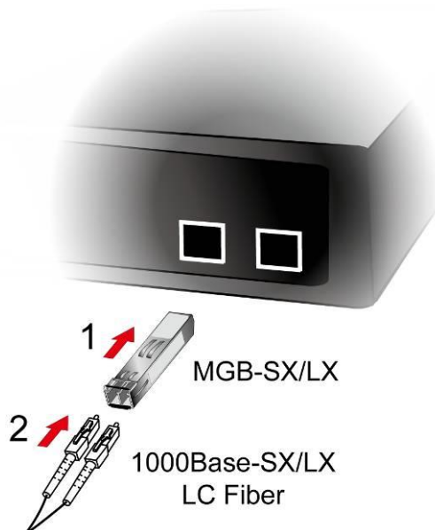
Figure 2-1-2c Plug in the SFP transceiver
