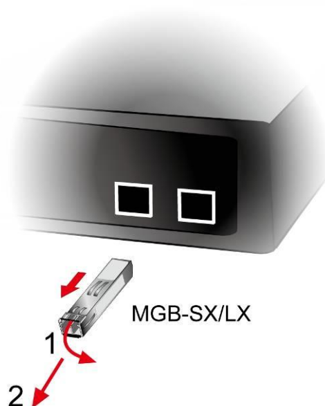
Figure 2-1-2d How to Pull Out the SFP Transceiver
