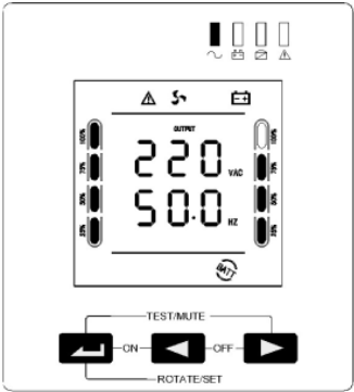
Figure 8. Screen with UPS control buttons
