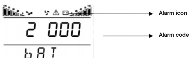
Figure 11. Error Code on the UPS Screen
