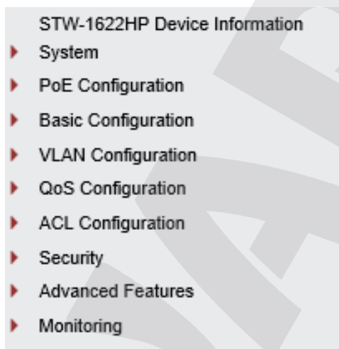
Figure 4-1-5: Web Smart Switch Main Functions Menu
