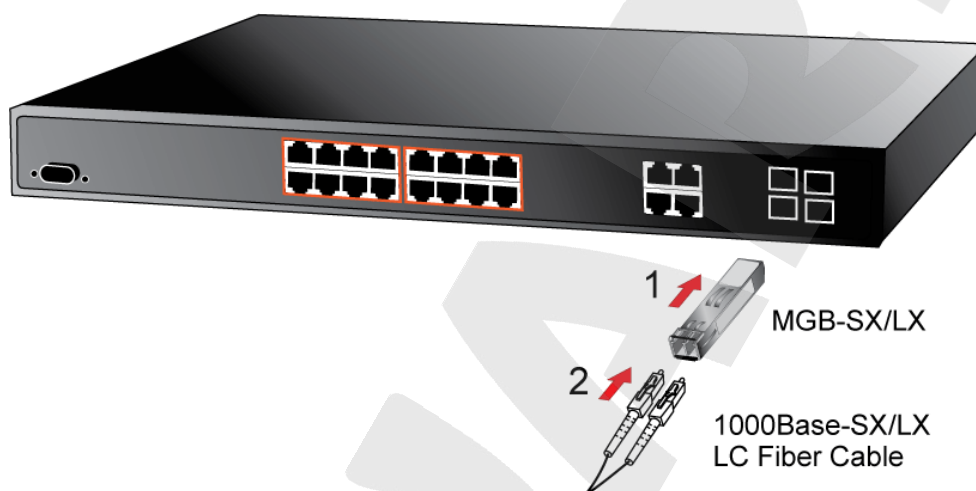
Figure 2-7: Plug-in the SFP Transceiver
