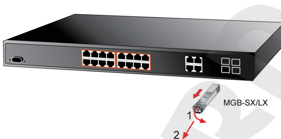
Figure 2-8: How to Pull Out the SFP Transceiver
