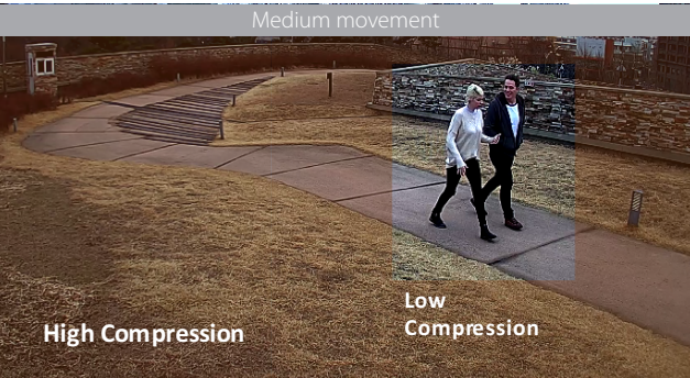
WiseStream II OFF : 7260kbps WiseStream II ON : 1817kbps
